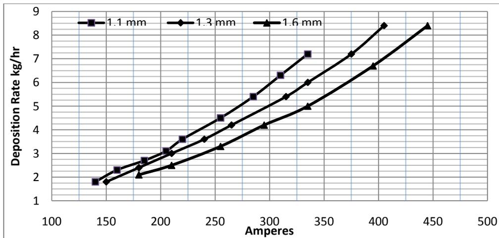
Figure 2 – Typical Deposition Rates for E491T-9-CH Consumables
