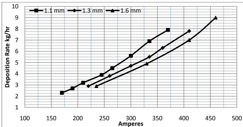
Figure 3 – Typical Deposition Rates for E492C-6-CH Consumables
