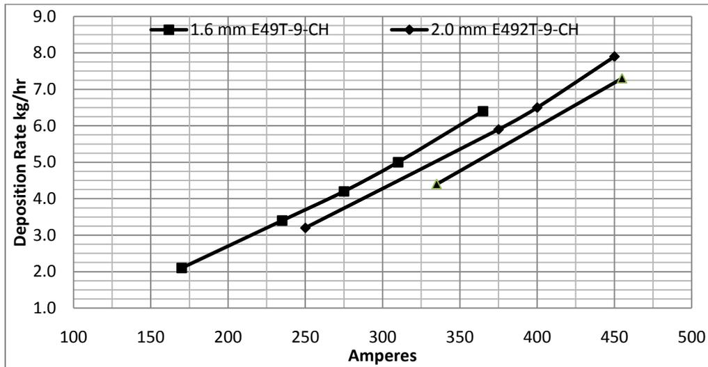
Figure 1 – Typical Deposition Rates for E492T-9-CH Consumables
